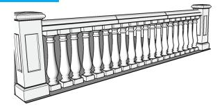
Finish the installation by grouting joints and patching any Imperfections/chips that may have happened during Installation. Wipe off excess grout with a wet sponge and keep the stone as clean as possible.
