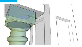
Repeat step #2 for each section of handrail. The final piece of handrail should be notched at the end, so the handrail sits on the dowel which is inserted into the newel post first. Now all you components are not only "glued" together, but mechanically fastened.
