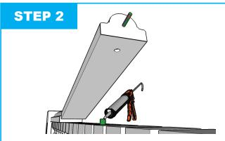
Each handrail should be doweled to one another following the same steps you did for the handrail to the newel post. Additionally, the handrail should be doweled to 1 baluster for each section of handrail.
