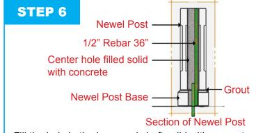
Fill the hole in the base and shaft solid with concrete and insert 1/2" rebar in filled hole through the base and shaft. *Tip: Grout joint between base & shaft prior to filling*
